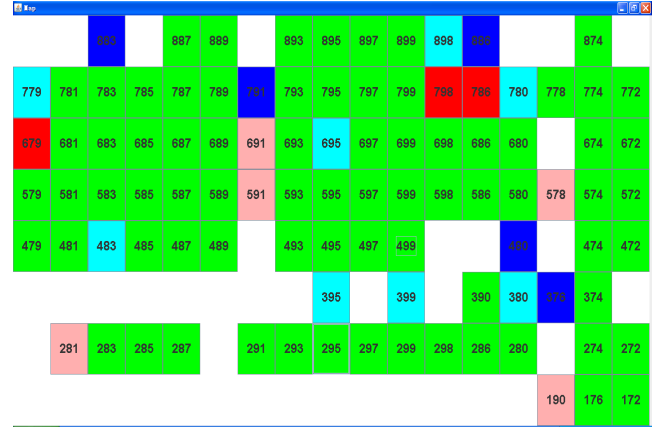
Figure 13. Room classification in Dreese building —Red: persistently hot; Blue: persistently cold; Pink: intermittently hot; Cyan: intermittently cold; Green: borderline and well-conditioned rooms.
