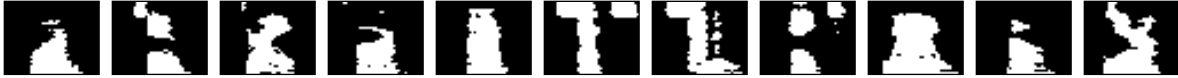
Figure 1: Typical ideal binary masks of isolated digit utterances 1-9, ‘oh’ and ‘zero’, ordered from left to right. In the figure, a white pixel indicates 1 and black pixel 0.
