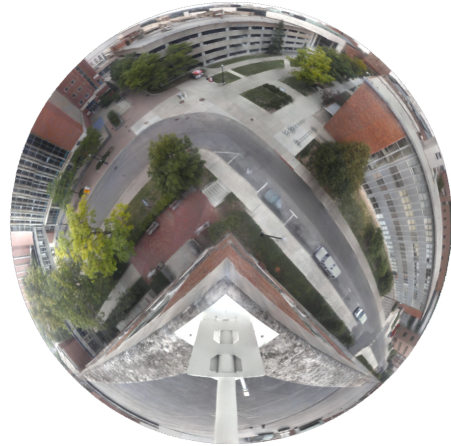
Figure 1. Spherical panorama representing the entire viewspace of a PTZ camera in a single image.
