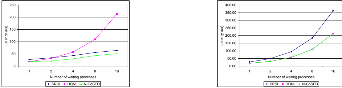
Figure 7. Lock Cascading Effect: (a) Shared Lock Cascade (b) Exclusive Lock Cascade
