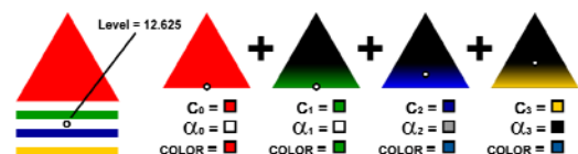
Figure 2. Diagram for implicit level determination
