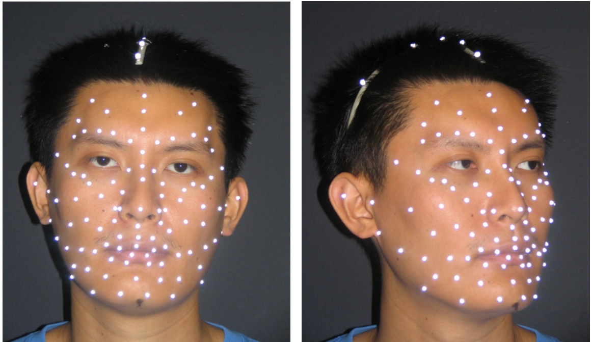
Figure 3.1: Front and side view of motion capture markers on skin and headband
