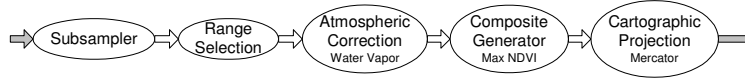
Figure 6: A high complexity Kronos query specified as a sequence of low-level functions. This query produces a data product transformed by a cartographic projection method.
