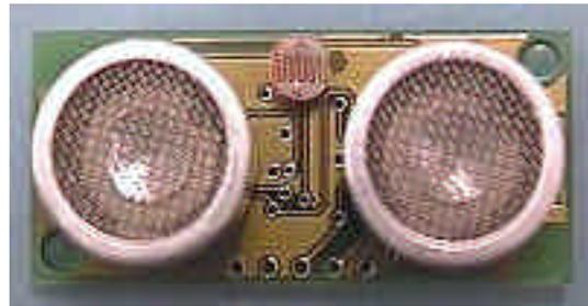
**Figure 4: Devantech SRF08 ultrasonic rangefinder.**
