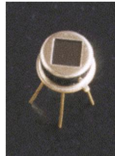
**Figure 8: Eltec 442-3 pyroelectric sensor with built-in signal conditioning.**
