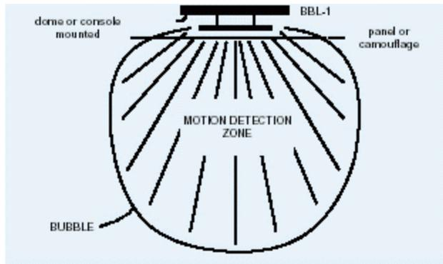
**Figure 7: Micropower impulse radar beam pattern.**
