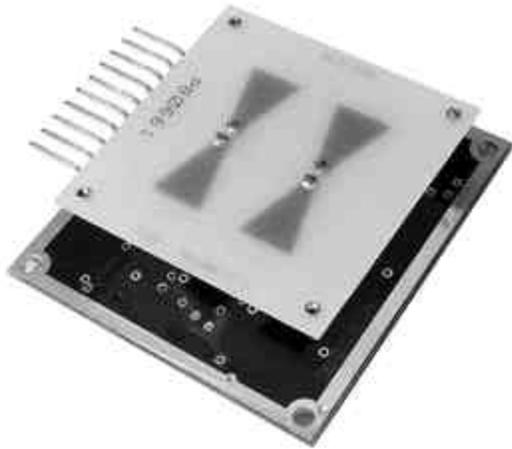
**Figure 6: Micropower impulse radar [10].**
