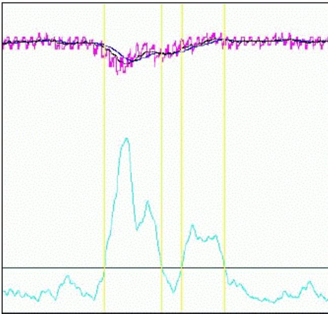
**Figure 3: Magnetometer signal detection and processing.** The purple signal is the raw signal, the dark blue is the raw signal after low pass filtering, and the light blue signal is dark blue signal after high pass filtering [7].
