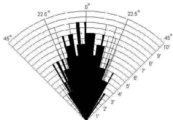
**Figure 5: Devantech SRF08 ultrasonic rangefinder's beam pattern.**
