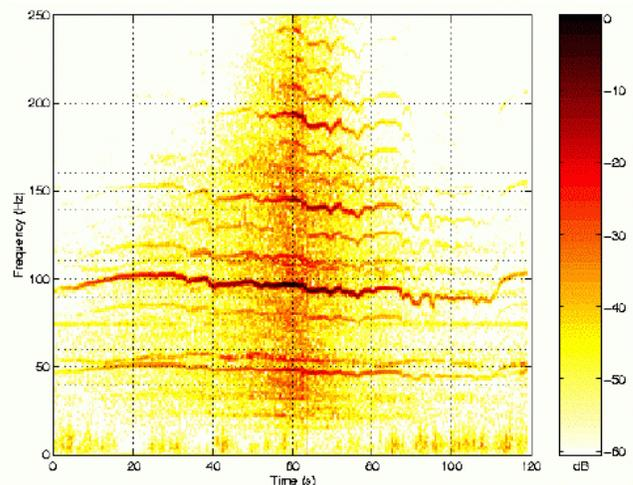
**Figure 2: Spectrogram of a tank traveling at a constant speed of 20 mph at Aberdeen Proving Ground (APG), MD [6].**
