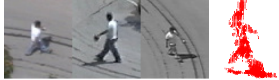
Figure 2. Three camera views of a person (left) and the resulting point cloud using VH reconstruction (right).
