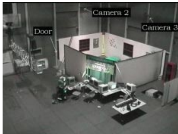
Figure 1: The KidsRoom is a 24 by 18 foot space constructed in our lab. Two walls resemble the walls in a real children’s room, complete with posters and windows. The other two walls are large back-projection screens. Six computers used to control the fully-automated room and additional audio and video equipment is located just outside one corner of the room. Computer-controlled lighting sits on a grid suspended above the space. The door to the space, where all room participants enter and exit, is pictured in the leftmost corner of the room.
