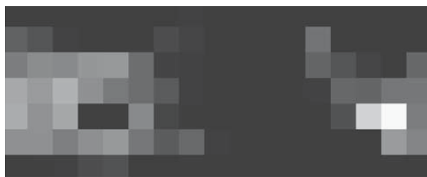
Fig. 8 A 7 \times 17 activity map (rows correspond to tilt positions and columns correspond to pan positions) after 10 complete passes of the scene, where brighter areas correspond to locations with more activity
