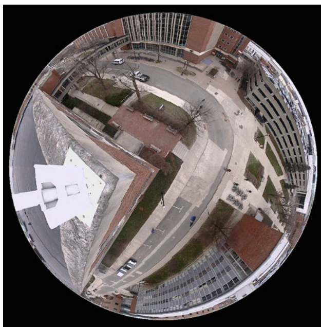
Fig. 11 Spherical panorama projection
