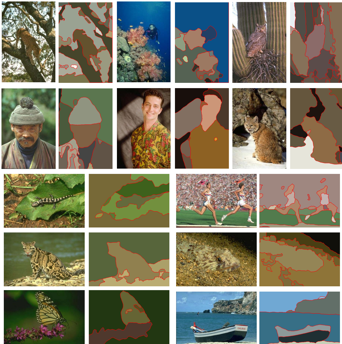
Fig. 6. Example results on Berkeley segmentation dataset. In each pair, the left is the original image, and the right the segmentation result from the proposed method, where each region is indicated by its mean color.
