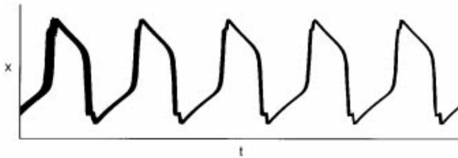
Figure 7: Synchronization in a 20 \times 20 2D network. The horizontal axis represents time, and the vertical axis x activity. The activity of all 400 oscillators is superimposed.
